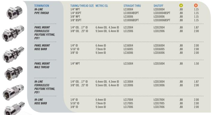
All measurements are in inches (millimeters) unless otherwise noted. Tubing must meet stated inside and outside diameters. †NOTE: CPC's Ferruleless Polytube Fitting terminations do not require ferrules to achieve a secure connection, which makes them easier to use and reuse. PTF fittings are designed for semi-rigid tubing, i.e., polyethylene, nylon, polyurethane, etc.
