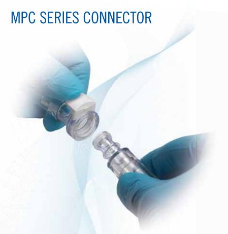
MPC Series couplings add ease of use and security to critical fluid handling applications. Choose from a full line of connectors and configurations, including pressure sealing caps and plugs, in sizes to fit 1/8" to 3/8" tubing. MPC couplings offer optional locking sleeves to further guard against accidental disconnects. In addition, coupling halves can be rotated when connected to reduce tube kinks.
