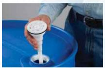
Place the drum insert assembly in drum.
