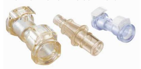
MPC/MPX Back-to-Back Adapters give end users the flexibility of connecting single-use systems that feature identical coupling connections at the end of their tubing. Combining both MPC and MPX couplings provides a reducing option for users who need to transition between tubing diameters ranging from 1/8" to 1/2".
