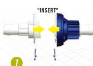
Align male and female connectors using the START alignment feature of the blue lock ring with the rib indicator of the white body. Insert the two halves together.
