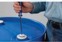
Turn shipping plug counterclockwise to remove. (Use a large, flat blade or #4 Phillips screwdriver.)
