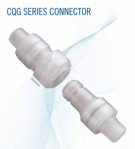
The CQG06 Series high purity couplings feature our patented pressurebalanced, non-spill design. Molded virgin polypropylene and a 100% springless flow path provide broad chemical resistance and exceptionally high flow capacity, allowing instant disconnects (and reconnects), even under pressure.
