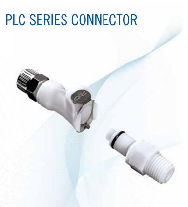
The 1/4" flow PLC Series is proven worldwide in thousands of applications and offers the widest selection of sizes and configurations. PLC couplings are injection molded from acetal thermoplastic and are resistant to most mild chemical solutions. One-hand connection/disconnection, plus integral terminations make the PLC Series the choice for ease of use and manufacture.
