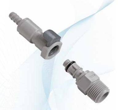
The 9/32" flow EFC12 Series couplings feature a high efficiency valve design that provides a greater flow capability than any other coupling its size. Chemically resistant polypropylene material makes it ideal for harsh environments. The EFC12 Series adds a bulkhead panel mount option for tight seals against tank walls and drums.
