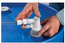
Turn the coupler locking ringclockwise until stop is reached (approximately 2 full turns); valve is opened during this process.
