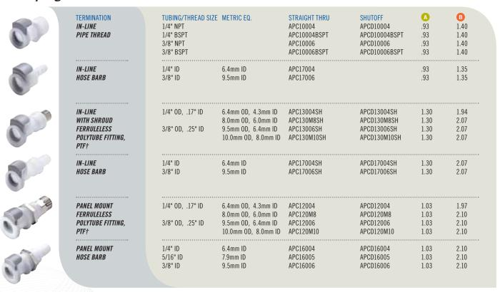
All measurements are in inches (millimeters) unless otherwise noted. Tubing must meet stated inside and outside diameters. †NOTE: CPC's Ferruleless Polytube Fitting terminations do not require ferrules to achieve a secure connection, which makes them easier to use and reuse. PTF fittings are designed for semi-rigid tubing, i.e., polyethylene, nylon, polyurethane, etc.
