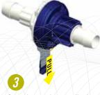
Snap the membrane pull tabs together and pull from connector.
