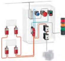
Guard Monitoring with Safety Module, Limit Switch, and Contactor
